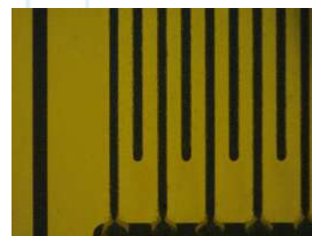
J-STD-004B Surface Insulation Resistance test showing no conductive anodic filament (CAF) migration or dendritic growth after 168 hours at 40°C, 90% relative humidity.
